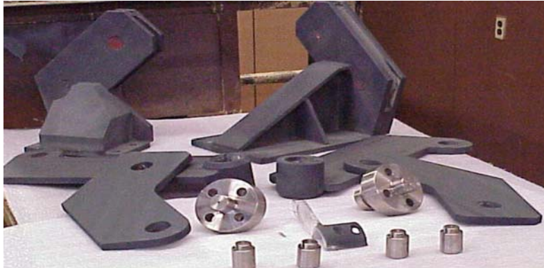
Figure 9: Example Parts Coated using the Nanostructure Plasma Sprayed material.
